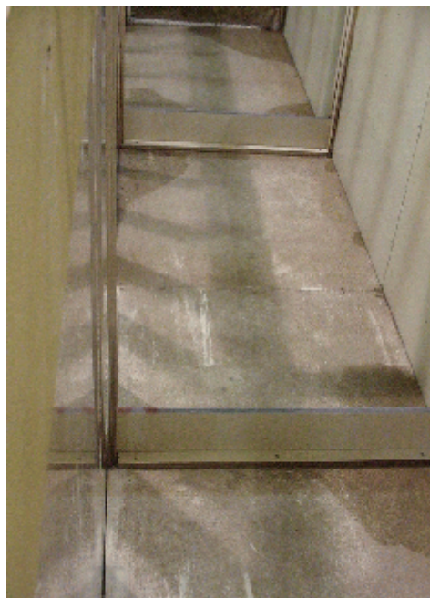
Figure 19 - View of 6 inch high weirs used to induce large scale vertical oriented eddies in the flow along the invert of the test flume.
